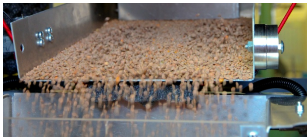
Figure 8. Shaker Tray with Counter Weight and Flowing Lentils.
