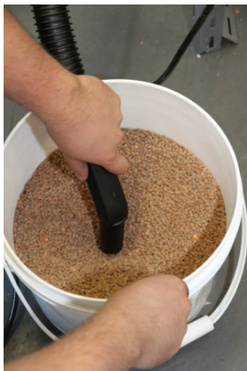
Figure 5. Lentils Being Sucked into Hopper.
