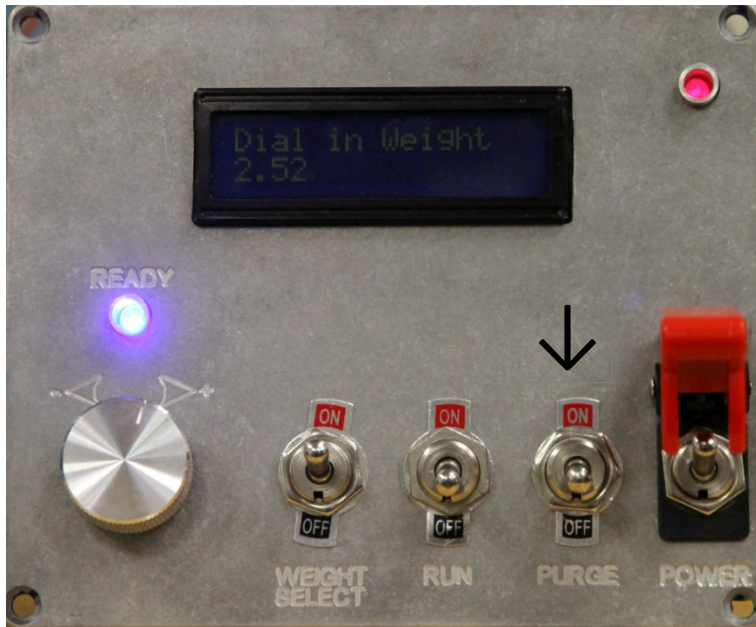
Figure 10. Location of the 'Purge' Switch on the Control Panel.
